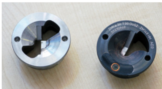
The integrated compact tag could be well protected in the cutting head (right)
