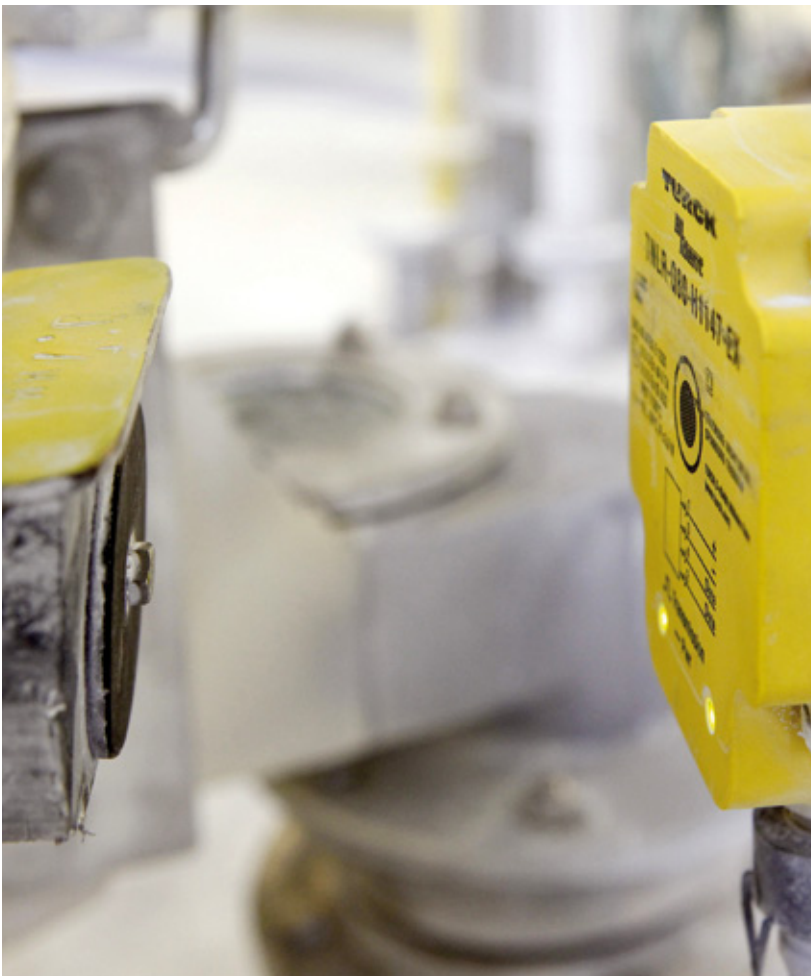
An Ex read/write head reads out the mesh width of the screen from the tag on the screen (left)
