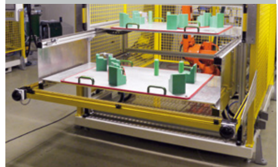
Intronyx protects robot cells for an automotive supplier with Banner Engineering EZ Screen safety light curtains from the Turck range. Page 24
