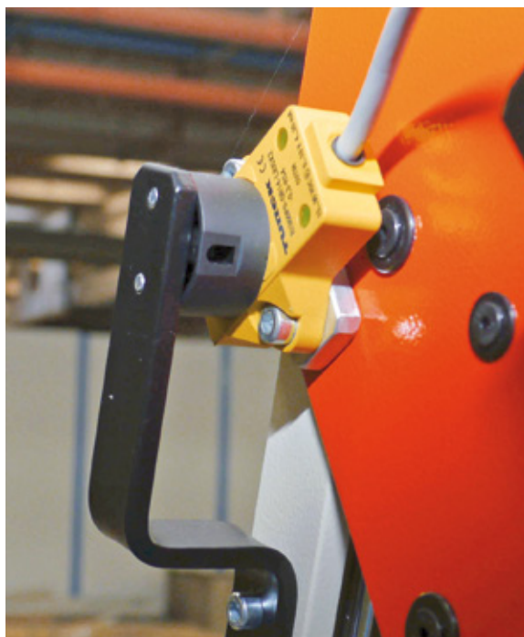
With a resolution of 0.09°, Turck's RI sensors provide more than sufficient accuracy
