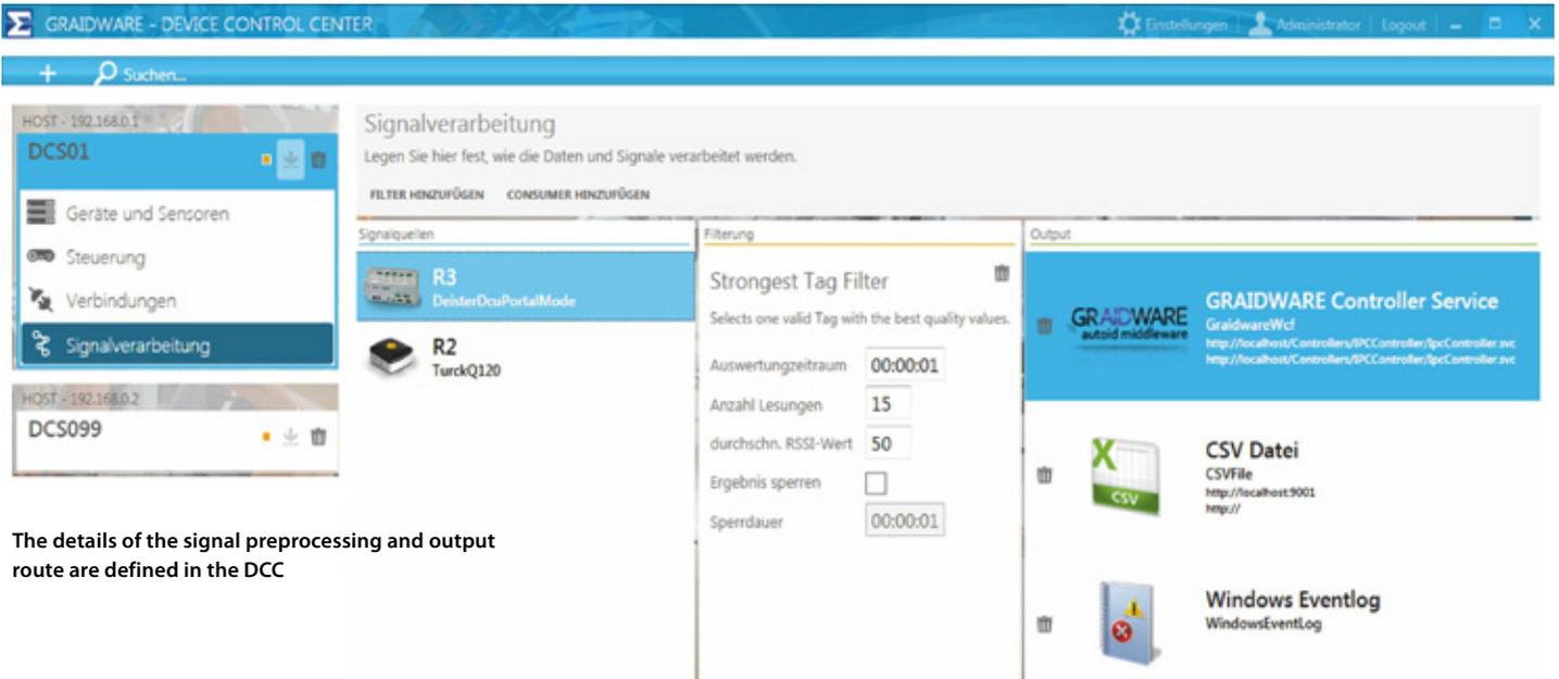
The details of the signal preprocessing and output route are defined in the DCC
