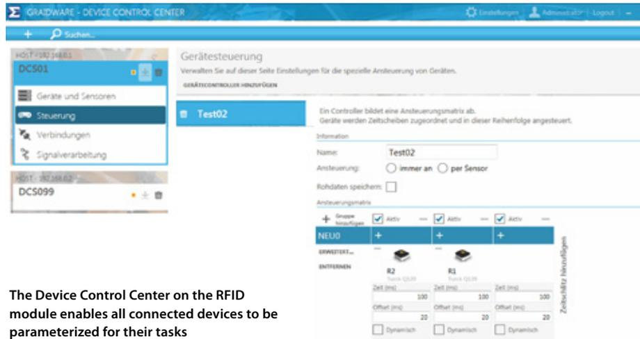
The Device Control Center on the RFID module enables all connected devices to be parameterized for their tasks
