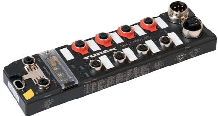
These devices can be used as remote safety I/O, or even operated as a standalone safety controller for local safe I/O; this allows the implementation of safety functions without the need for a safety PLC while still providing safety diagnostics and general purpose I/O data to a higher level non-safety PLC.
