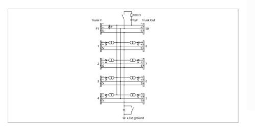
The 8-channel junction box EG-VA2020/ BV68-T085/JRBS-40SC-8C/EX is designed for FOUNDATION™ fieldbus systems.
