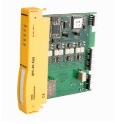
The DPC system (Diagnostic Power Conditioner) is a power supply system for the installation of FOUNDATION™ fieldbus H1 segments. It provides extensive diagnostic options for monitoring FOUNDATION™ fieldbus segments and thus supports plantwide asset management.
