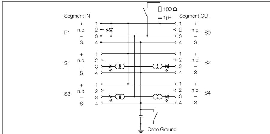
The 4-channel Ex junction box JBBS-48SC-M413/EX is designed for PROFIBUS-PA systems.
