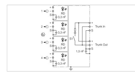
The 4-channel multibarrier MBD48-T415/EX enables the connection of a large number of field devices to one fieldbus in the Ex-area, according to IEC 61158-2.
