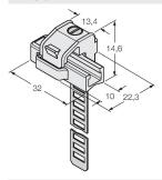
Mounting bracket for mounting magnetic field sensors on round cylinders; cylinder diameter: 130...250 mm; material: PA 6I/6T / nickel silver; fire-hazard classification acc. to UL94 -
