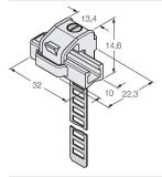
Mounting bracket for mounting magnetic field sensors on round cylinders; cylinder diameter: 25...63 mm; material: PA 6I/6T / nickel silver; fire-hazard classification acc. to UL94 -
