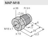
Mounting adapter; material: Polypropylene; sensor replacement with filled container possible (adapter remains in container during sensor replacement)
