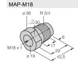
Mounting adapter; material: Polypropylene; sensor replacement with filled container possible (adapter remains in container during sensor replacement)
