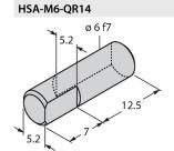
Adapter for RI-QR14 specific positioning elements, hollow on solid shaft, Ø 6 mm
