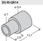
1590814 Spacer sleeves for rear mounting of RI-QR14, 2 pcs. per bag
