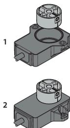
There are two different mounting options. One option is to position the positioning element above the sensor housing. However, it can also be mounted so that the sensor housing completely encloses the positioning element.
