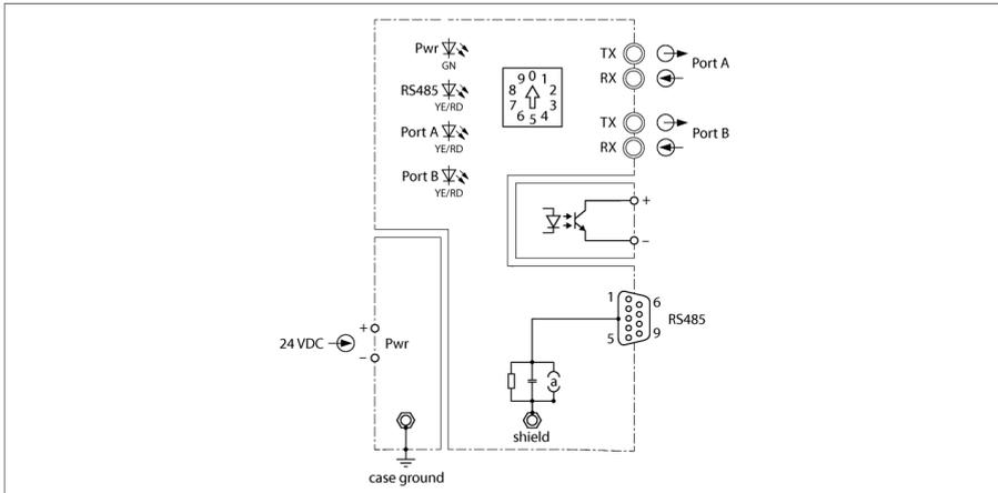
The FOC12... fiber optic media converter converts RS485 signals, e.g. from PROFIBUS-DP or Modbus RTU, on copper cables into optical signals and vice versa. The bus signals can therefore be transmitted from the safe area up to Zone 1 over long distances in a way that is intrinsically safe without potential or interference.
