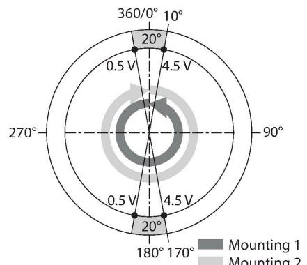
There are two different mounting options. One option is to position the positioning element above the sensor housing. However, it can also be mounted so that the sensor housing completely encloses the positioning element.
