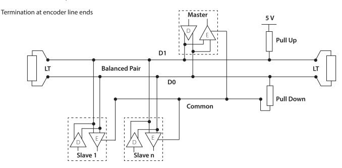
The bus termination is software configured by means of a register value. Once the Modbus has been looped through, it must be terminated between D0 and D1 at both ends using 120 ohm bus termination resistors on the last device.
