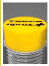
Unique mounting flexibility of *uprox*°+ sensors is achieved with embedded pre-damping protection. In contrast to conventional sensors with a ferrite core, free zones can be much smaller. Nonflush threaded barrel sensors can be mounted up to the edge of the thread with reduced switching distance.
