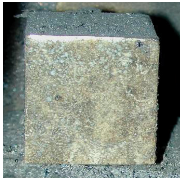
Turck Weldguard lasted 25,691 welds.
