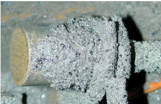
Competitors failed at less than 2,000 welds. Turck Weldguard lasted 34,256 welds.
