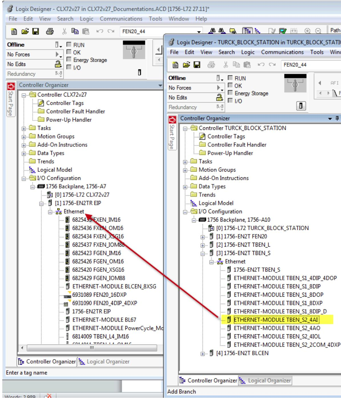
2. Highlight the “ETHERNET-MODULE TBEN\_S2\_4AI” in the Controller organizer of the project and open “Module Properties” page. Assign IP address; name can be changed as well. Click Apply and OK.
