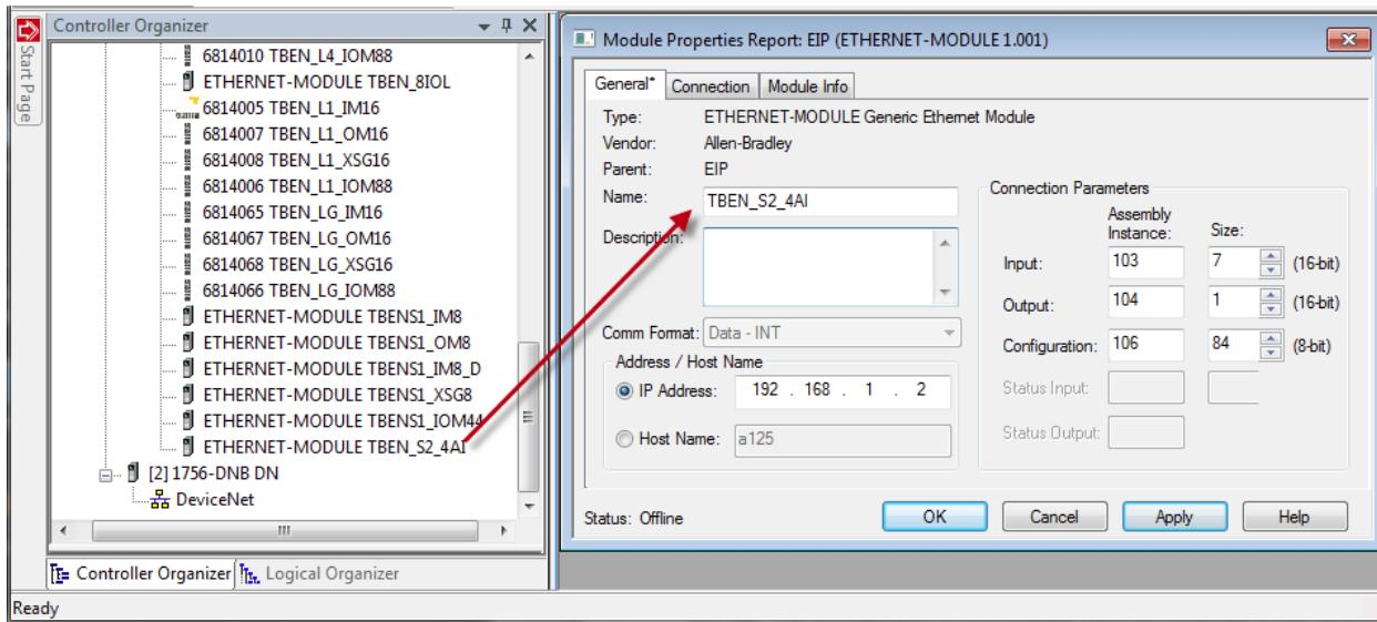
The controller creates configuration tag, input tag and output tag. It also saves content of the configuration tag. The configuration is downloaded from the controller to the device every time when device is connected to the controller.
