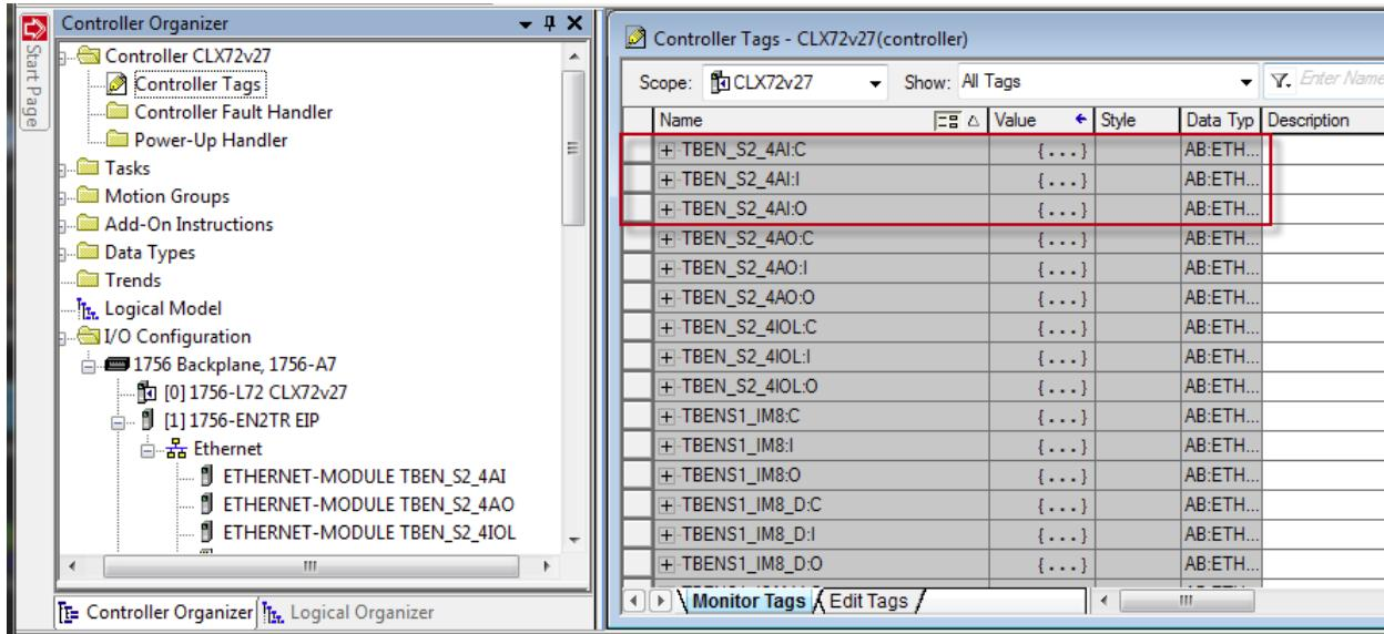
TBEN-S2-4AI is universal analog input device. It supports multiple analog signal inputs such as: thermocouple input, voltage or current inputs, resistance or RTD inputs. 4 analog input channels may be set to different mode of operation which has dedicated set of configuration parameters. These are contained in the configuration tag.
