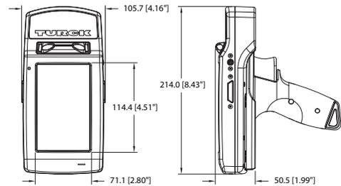
Fig. 2: Scale drawing– Device with grip handle
