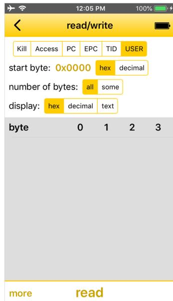
Fig. 6: Turck RFID app – Screen: Read/Write
