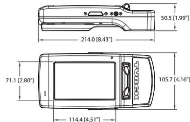
Fig. 1: Scale drawing – Device without grip handle
