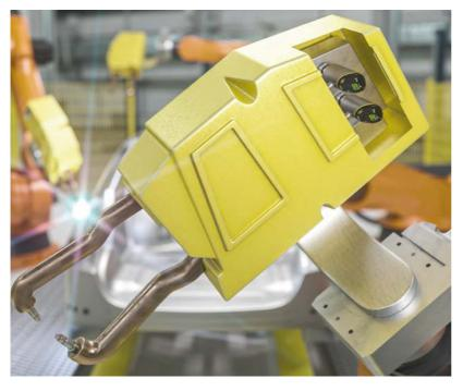
Monitoring the cooling circuit on welding clamps
