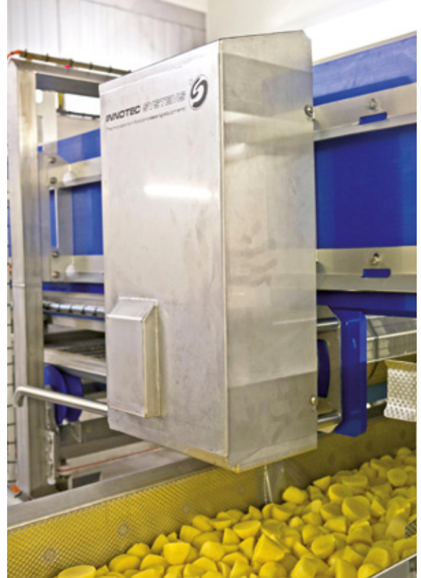
Double protection: The stainless steel guard covers the entire motor together with the encoder during operation
