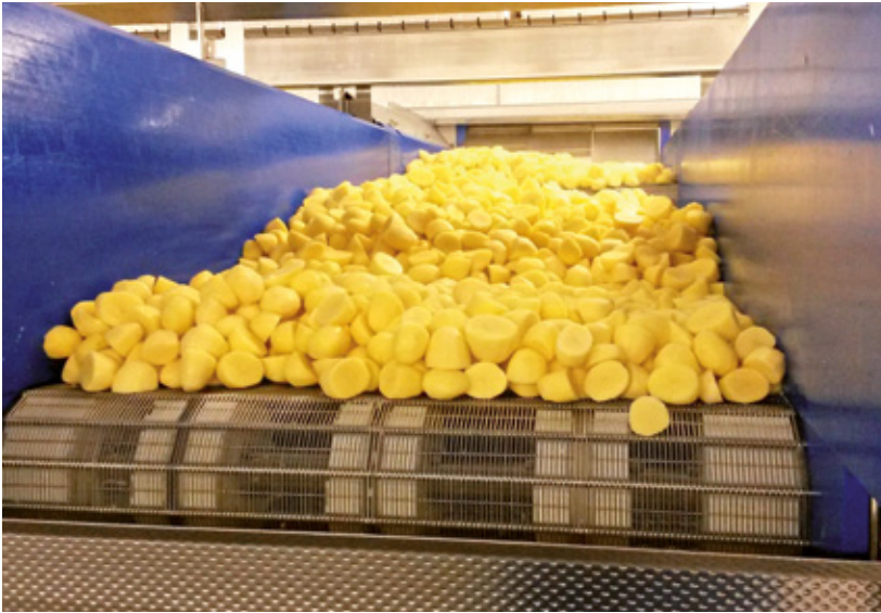
Buffer conveyor: Up to 500 kilos of potatoes can be buffered on both belts
