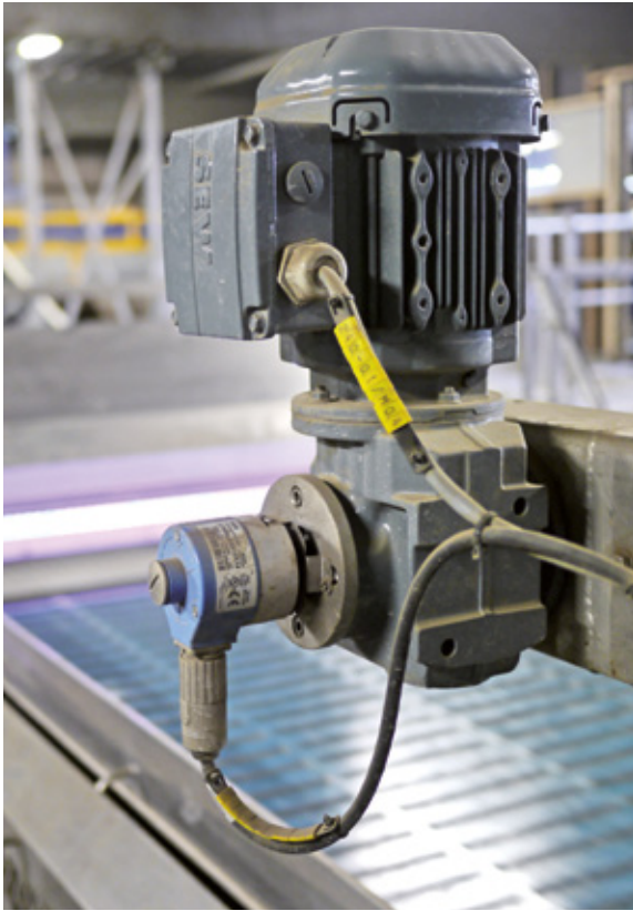
Previous solution: The spring mounting of this encoder was susceptible to mechanical faults and wear
