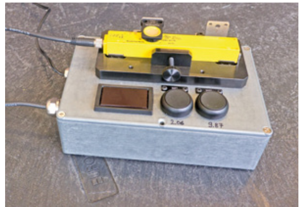
Precitrame built this device itself to enable its employees to teach the Li sensors the required 55 millimeter measuring range at the push of a button
